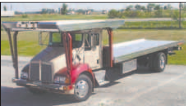
KENWORTH T300 Featuring 315 hp, 10-speed transmission, Chevron 28' aluminum 4-car carrier.
