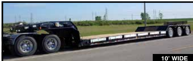
NEW 2014 ETNYRE BLACKHAWK AGRICULTURAL TRANSPORT TRAILER triaxle, 40 ton, 10' wide, aluminum pullouts to 14' wide, air ride, 60" spread, 25 ton hyd winch, hyd detach PLACE YOUR ORDERS
