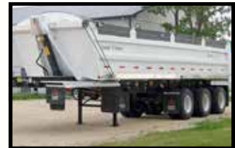
NEW 2013 CANUCK END DUMP R3 - Hardox 450, tub, 60" spread, air ride, asphalt overhang, electric tarp 2 IN STOCK
