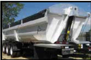
NEW 2014 NORTH COUNTRY END DUMP , triaxles & tandems available, Hardox 450, HT 300 air ride susp, 60" spread, $56,500
