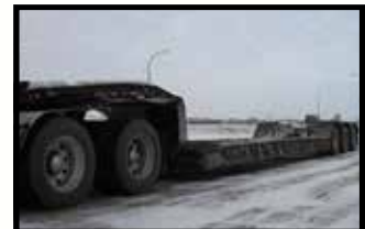
2003 TRAIL KING 50 TON DD LOWBED , triaxle, hyd detach, air ride, 55" spread, 8'6" wide, c/w swingouts, fenders, mint, safetied, $42,500 OBO
