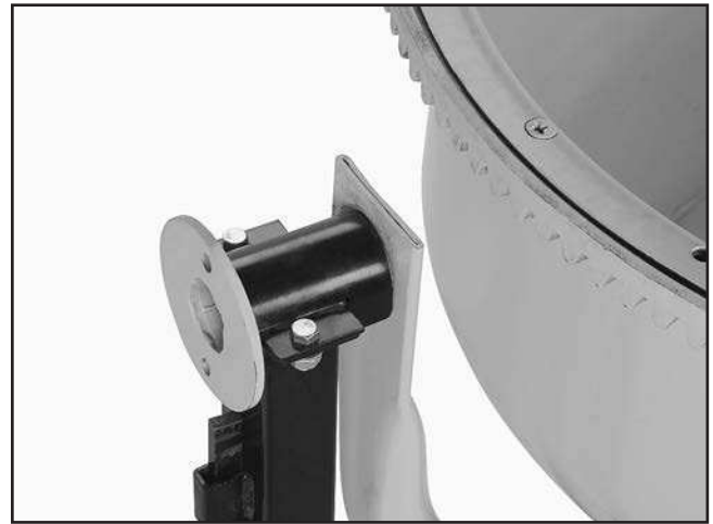
Figure 10. Upper bracket installed.
