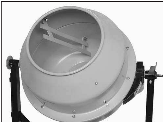
Figure 13. Upper part of mixing blades attached to upper drum.
