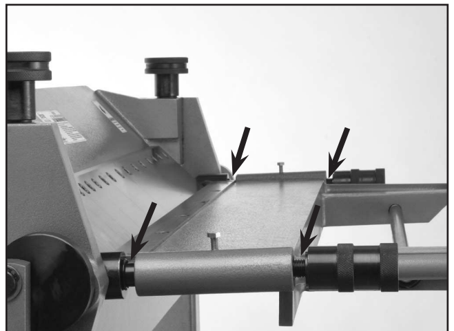
Figure 23. Location to lubricate setback threads.
