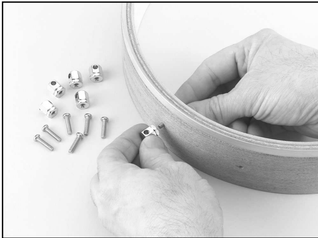
Figure 4. Installing the bracket hook lugs.
