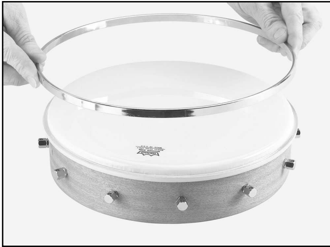
Figure 6. Installing the tension hoop.
