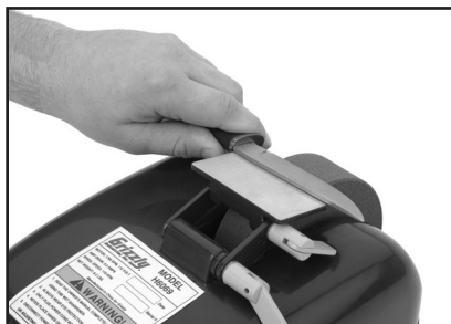
Figure 4. Correct positioning on tool rest.
