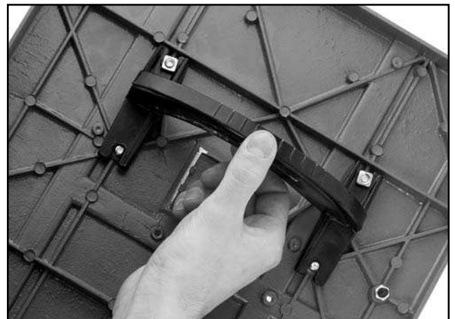
Figure 11. Sliding the trunnion onto the table.
