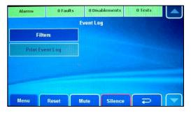
To either filter, or print, the log press one of the blue event log buttons and the window shown left is displayed:
