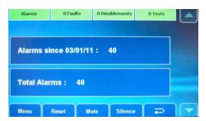
The display will show the total number of times the panel has been in an alarm condition since it was last cleared (upper button) AND the total number of alarms from its installation date (lower button).
