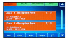
If more than one device is in a fire condition on the zone, the top right corner of the display will show, for example "1 / 3" and can be scrolled through using the \( \subseteq \) and buttons, or by using the scroll bar.
