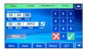
Adjust the time and date using the touchscreen's numeric keypad and buttons. Also, set/unset the daylight saving time by pressing the **DST** tick box.
