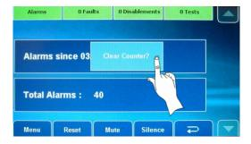
Press the button to return to the main access level 2 menu, or to clear the alarm counter press the 'upper' blue button. A small **Clear Counter?** button will appear (shown above right). (Note that the Total Alarms counter cannot be reset.)
