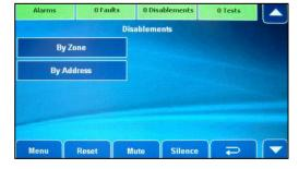
Press the **By Zone** button to select and disable <u>all</u> devices within a specific zone, or press the **By Address** button to select and disable individual devices by entering their loop number and address.
