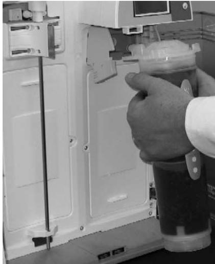
**Quantum Cartridge being placed into the pack adapter.**
