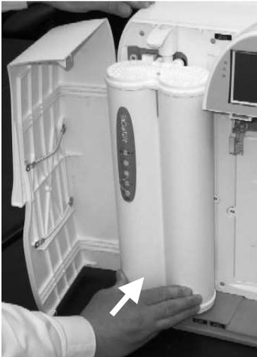
**Pak Locking Handle being pushed down while holding the bottom of the Q-Gard Pack.**
