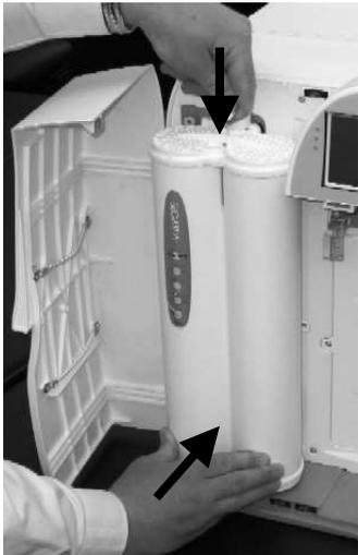
**Section 3-8 QUANTUM CARTRIDGE INSTALLATION**
