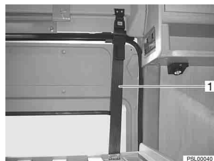
Fig. 38 Retaining strap pull-down bed
