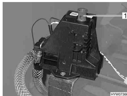
Fig. 58 Safety/drainage valve of the boiler
