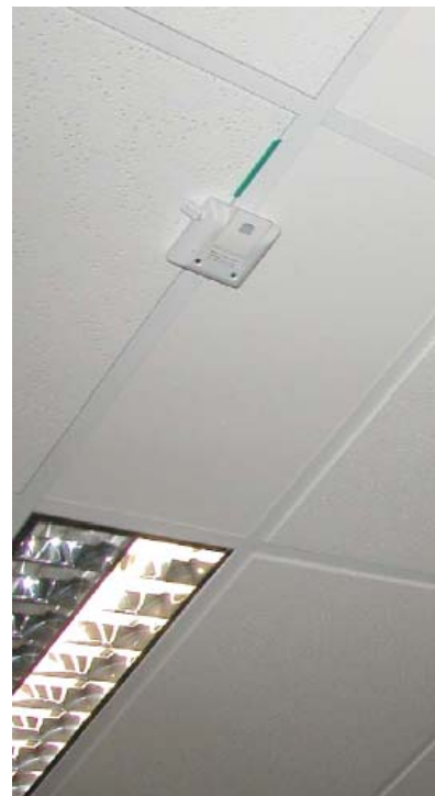
Figure 15: Occupancy/light status logger
