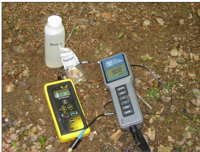
Figure C2: Bacteria sampling materials (clockwise from top: 16 oz. HDPE sample bottle, Whirl-pak® bag, YSI 85 meter, and handheld pH meter)
