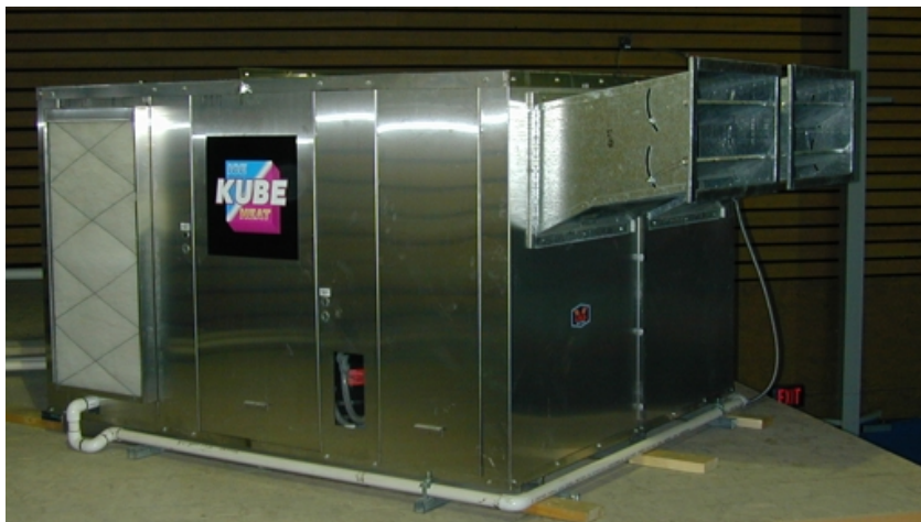
Figure 1. Eight low temperature water-to-water heat pumps provide approximately 84 tons of refrigeration at ice rink temperatures. The heat pumps reject heat either directly to a radiant floor heat system or to a horizontal earth loop.
