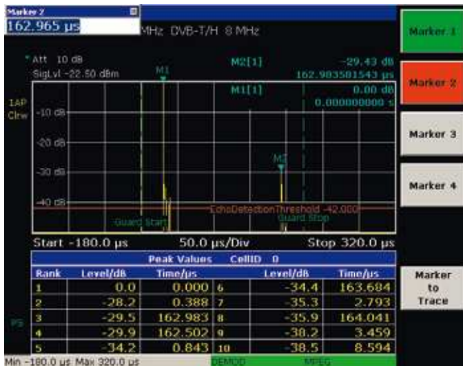
DVB-T, DVB-H channel impulse response with markers.
