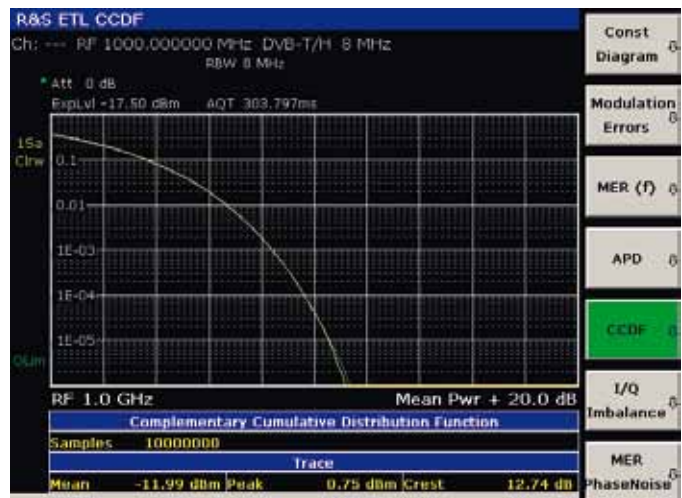
Complementary cumulative distribution function (CCDF) measurement.
