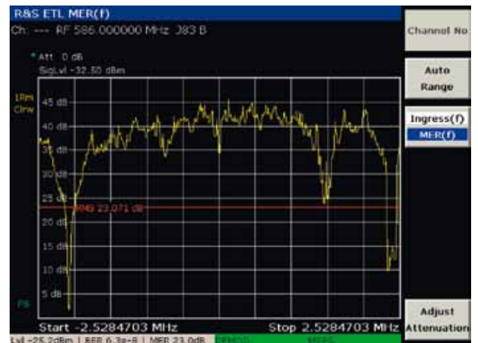
MER (f) of a J.83/B-signal with superimposed interfering.
