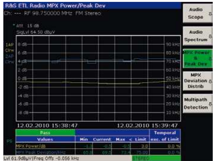
MPX deviation and MPX deviation distribution.
