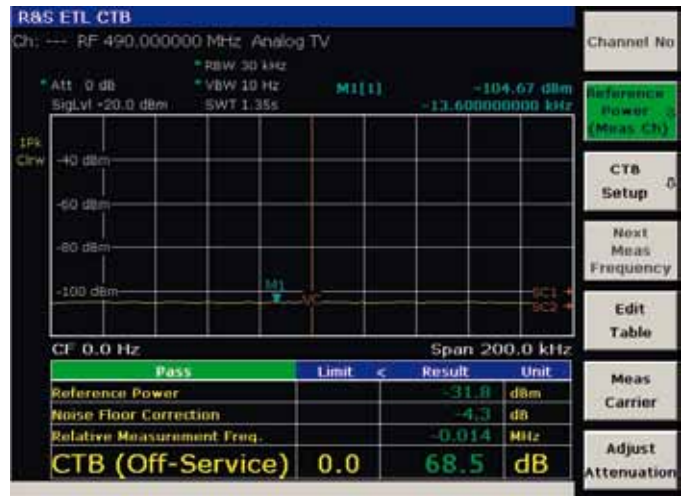
Composite triple beat (CTB) measurement.
