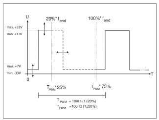
If no signal is present the pump accelerates up to its final rotation speed.
