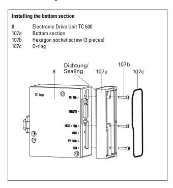
→ First pull the corresponding cables through the inserts with screwed cable glands and the cover 107d and insert the cables at the TC 600.
