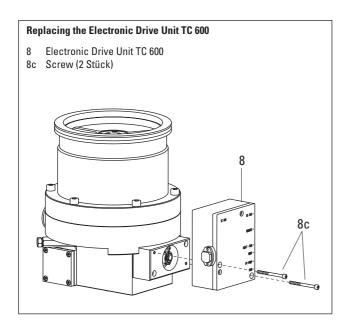
→ Install the new Electronic Drive Unit TC 600 back onto the turbopump and connect again.
