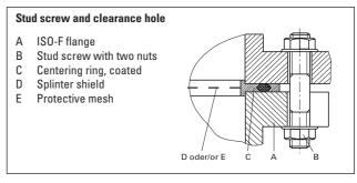
→ For a flange material having a strength of > 170 N/mm² and a stud screw with clearance hole, the nuts must be tightened crosswise in three steps.
