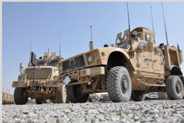
This MRAP platform used by the Marine Corps is produced with high-strength armor steel to extend its life cycle. Photo courtesy of the U.S. Marine Corps.
