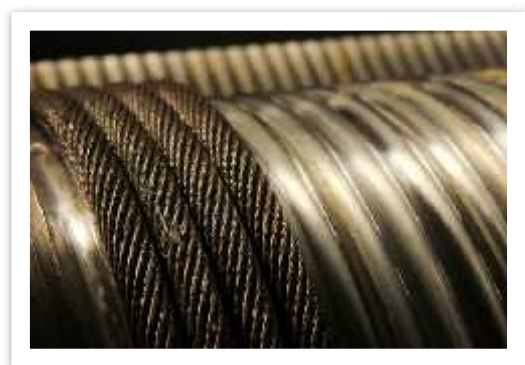
Neither the load nor the boom must be lowered below the point where less than two full wraps of rope remain on their respective drums.
