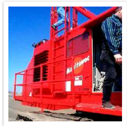
Equipment must be equipped to provide safe access and egress between the ground and the operator work station(s).
