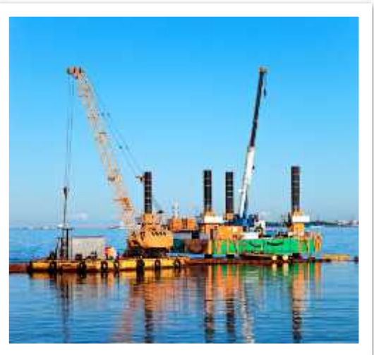
The rated capacity of land cranes/derricks on floatation devices must be reduced to take into account the additional instability.
