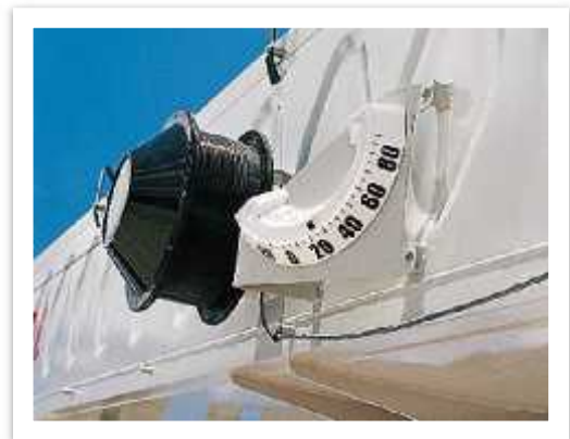
A boom angle is required on all luffing boom tower cranes and hammerhead tower cranes manufactured after November 8, 2011.
