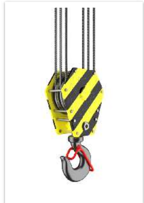
New hoists must be load tested to a minimum of 110% capacity, but not more than 125% rated capacity.
