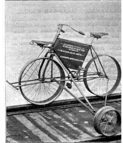
Fig. 2. New Track Velocipede with Toolbox and Extra Seat Attached.
