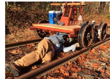
Me checking axle box nuts for tightness en route.
