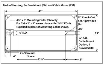
Order SM ceiling type. Mounting collar required for surface mounting. (4) Mounting knock-outs, 3/8", provided in center channel as indicated at left, marked "A". **Cable Mount:** Order CM ceiling type. Use CM48Y2SC3F-KIT 48" Cable Mount Kit for 2' wide SM trim fixtures. Mounting holes are provided in diagonal straps shown at left, marked "B".
