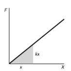
You also saw previously that the work done by a force can be calculated from the area under the force vs. position graph. Shown below is a plot of the magnitude of the force (F) vs. position (x) for a spring. Note that k is the *slope* of this graph.
