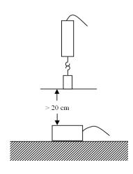
In this activity you will measure the work done when you lift an object from the floor through a measured distance. You will use the force probe to measure the force and the motion detector to measure distance.
