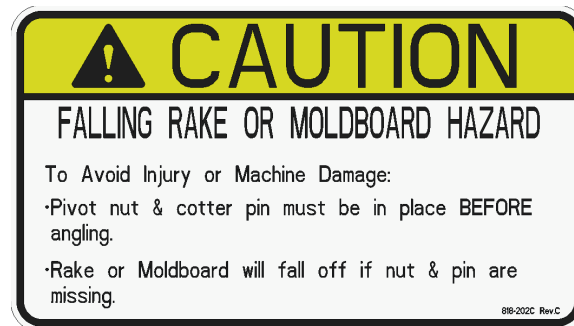
818-202C Caution: Falling rake - Retaining hardware
