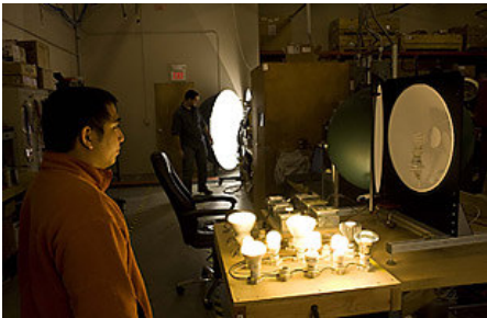
Lightbulbs in integrating spheres at the Electric Power Research Institute are tested for energy consumption and longevity Jeff Jacobson / Redux for TIME
