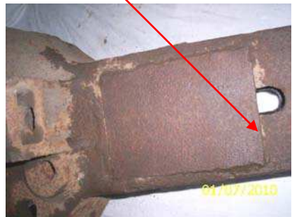
Condemning limit of shank wear plate
