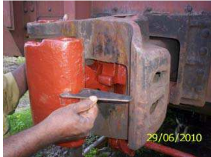
Wrong practice of gauging
