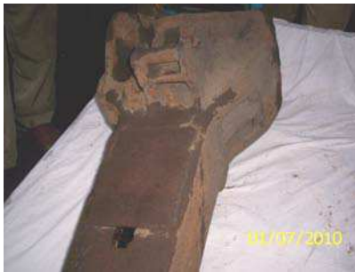
View of new shank wear plate
