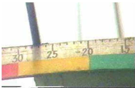
Fig-22 Mainline stagger of turn out OHE should not exceed than 300 mm
