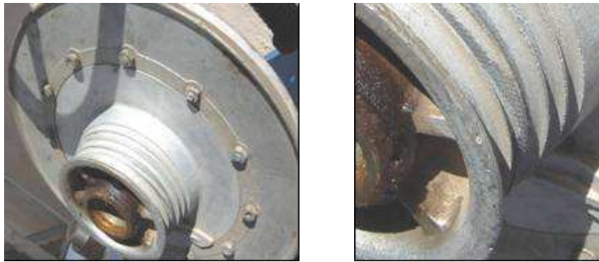
Fig- 26 Checking for damage of groove using GO - NO -GO Gauge
