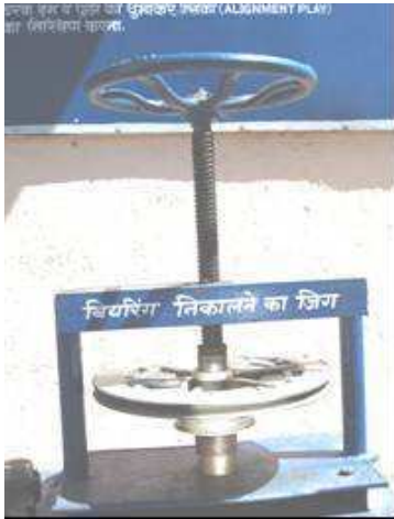
Fig-29 Bearing jig and damaged housing & bearings
