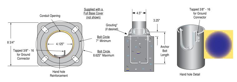
NOTE: Factory supplied template <u>MUST</u> be used when setting anchor bolts. Philips Gardco will not honor any claim for incorrect anchorage placement from failure to use factory supplied templates. \* Grouting should include a drainage slot or tube (by others) to permit water to drain from the base of the pole. Failure to provide drainage may weaken the pole base structure over time and may result in pole base failure, for which Philips Gardco is not responsible.
