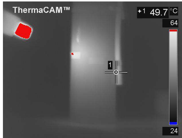
Figure 4. - Infrared picture of an ABC fire extinguisher while being heated with a heat gun. The white square areas on the extinguisher are black electrical tape.
