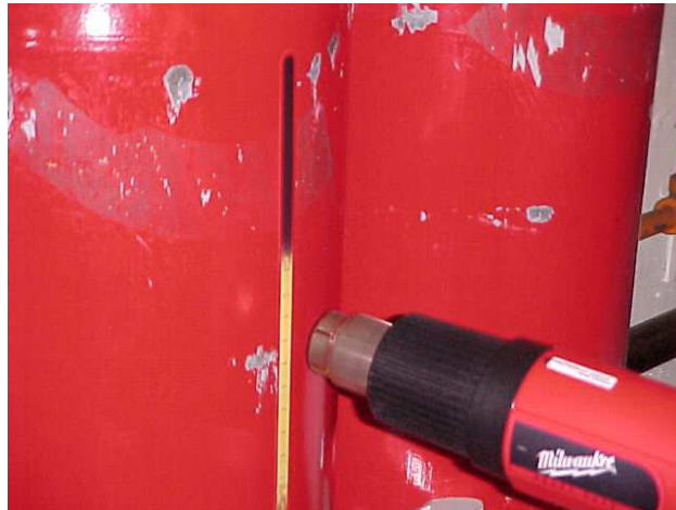
Figure 1. - Heating Liquid Level Strip
