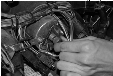
Remove speedo cable/unplug gauges
