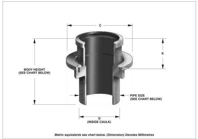
Note: The R1854 is made out of lacquered cast iron material. All other sizes are made from fabricated 14 gauge galvanized steel that is powder, epoxy coated with an electro-static application. These models are standard with an acid resistant epoxy finish.
