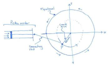
To make her calculations easier, she drew a coordinate axes with origin at the center of the flywheel, and she labeled the joint where the crank arm attaches to the connecting rod by the point P. As part of the design specifications, the crank arm is 60 cm in length, and the motor spins the flywheel at a constant rate of 100 revolutions per minute.
