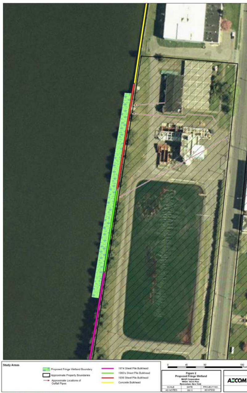
Figure 2. Bulkhead Enhancement Plan View
