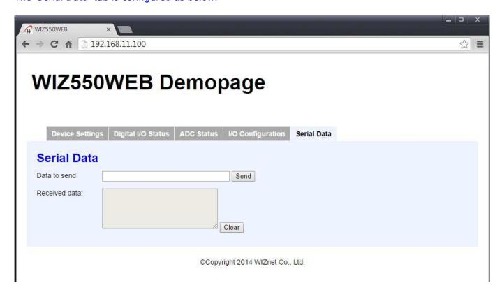
In this page, user can test the 'Serial data input/output through Webpage to UART1' (Serial data Tx/Rx) functions.
