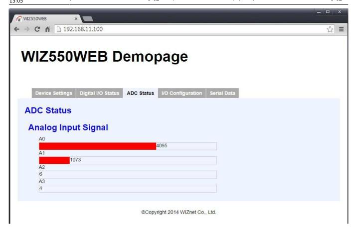
The Analog input signal through ADC changes into a bar graphs is displayed in real-time.
