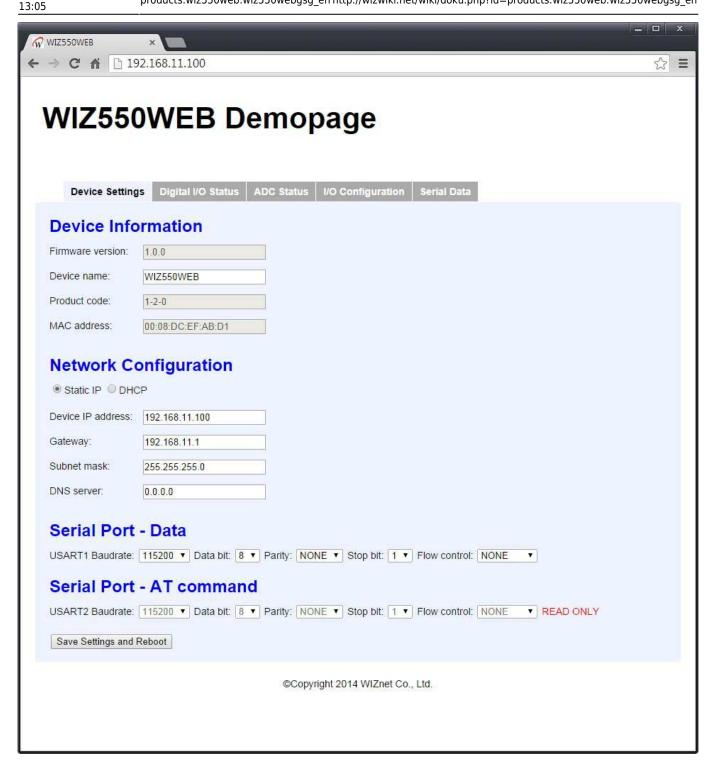
The user can check the device information like MAC address / Firmware version and set the network information (IP address, DHCP options and etc.), serial port configuration through the 'Device Settings' tab. After adjusting the settings, if the **[Save Settings and Reboot]** button is pressed, the configurations is saved and the WIZ550web module reboots. Please note that the module is rebooted after the settings.
