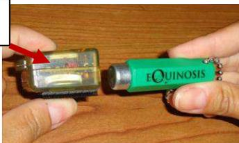
Each Lameness Locator® sensor is designed with an automatic “power-off” feature. The sensor will automatically shut off if not connected to the Lameness Locator® software after 20-30 minutes, depending on existing battery charge. This functionality is designed to spare battery power if the user inadvertently forgets to shut off the sensors after use.
