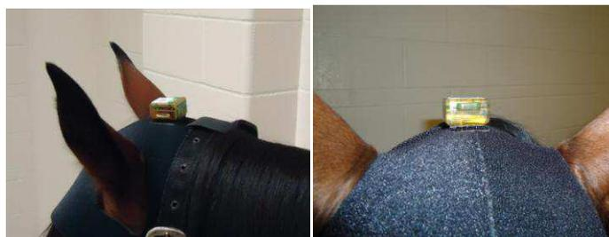
Also, attaching the head sensor to the Lameness Locator® felt head bumper reduces wiggle and noise from the head sensor during data collection. While attached to the head bumper, the sensor will move more reliably in better synchrony with the entire head. The head sensor is simply “snapped” onto the
