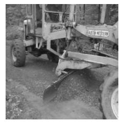
**Preparing the Road.** Before you place the aggregate, or before you apply a dust suppressant for that matter, you must perform routine maintenance on the road and, if necessary,
