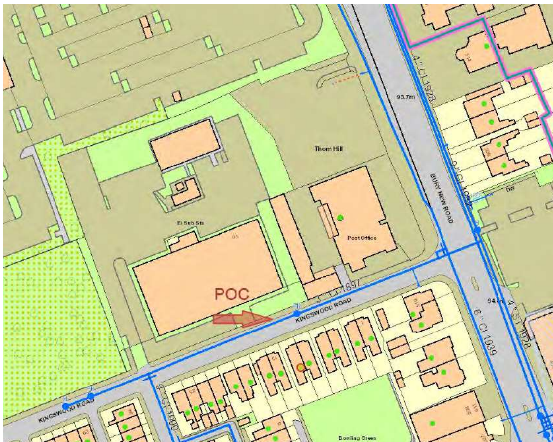
Figure 4.2 United Utilities Point of Connection
