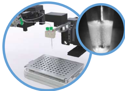
Fig. 1.6. QX200 droplet reader autosampler.
