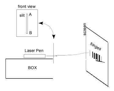
The laser light you have used for the SOL experiment can be viewed either as a wave or as a stream of photons (quanta of energy). When light interacts with objects that are comparable to its wavelength, it can behave in very counterintuitive ways. This experiment is designed to illustrate this.
