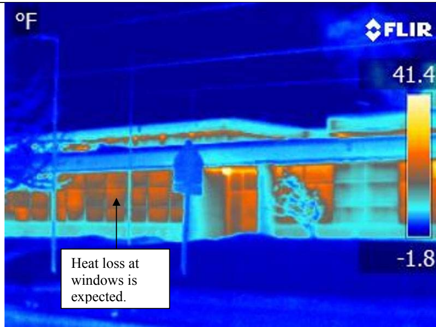
2. Thermographic Image, Main Entrance. No unusual heat loss observed. Temperatures indicated by color scale on right. Yellow indicates heat leakage. The outside temperature was about -14°F.
