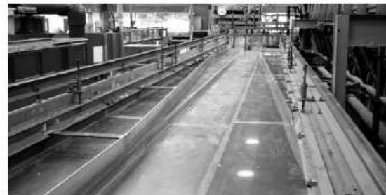
Figure 2. Photograph of the University of Birmingham's experimental flume with a skewed geometry
