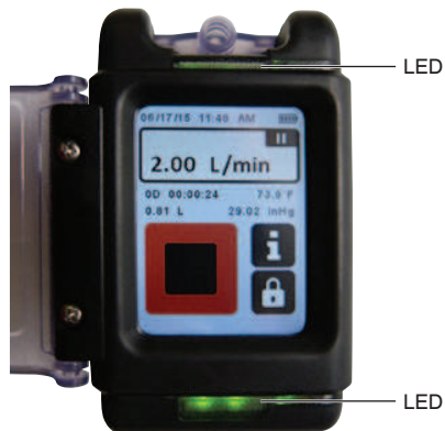
Figure 5. Green, flashing = Pump or schedule running
