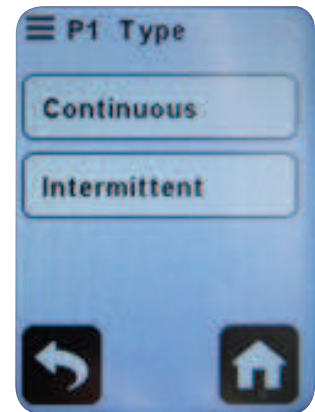
3.b a. To program a continuous sample: Touch Continuous b. To program an intermittent sample: Touch Intermittent
