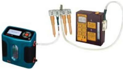
Connect holder to pump intake and tube inlet to calibrator.
