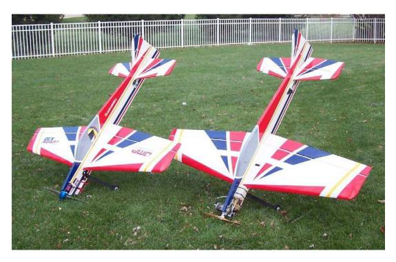
Wingspan: 70" Wing Area: 1045 sq. in. Length: 69.5" Approx. Weight: 7.25-7.75 lbs. Engine: 1.20 glow, 20 cc gas E50-E60 motor with 1900-2100 Watts
