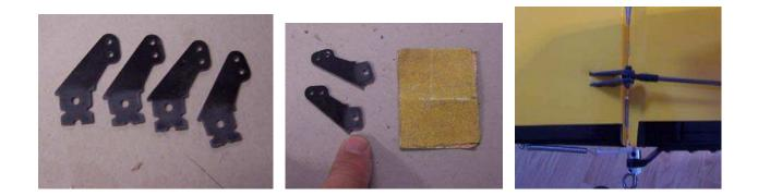
3. Locate the parts for the main landing gear. Two guide holes are provided in the fuselage for mounting the main landing gear. Cut the covering away from these holes and mount the main landing gear using the supplied bolts, washers, and lock nuts. Mount the wheels to the main gear by installing the supplied bolt (bolt has a smooth shank on it) into the wheel, installing a nut on the bolt (tighten just enough to allow the
