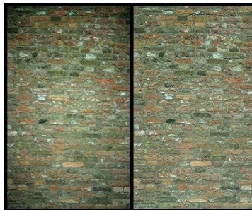
Figure 4.4 Vignetting seen in a photograph for two aperture sizes. Left: f/1.4 . Right: f/5.6 [29].
