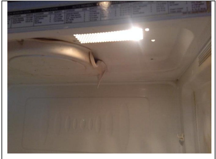
Sample of melted components in the microwave
