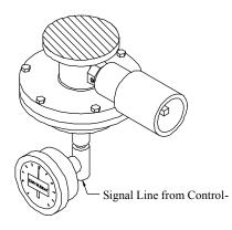
6. If the actuator is equipped with an MCV-3 Manual Control Valve), place the left MCV-3 handle in the manual position. If the actuator is not equipped with an MCV-3, use the block valve (1/4 " ball valve) installed between the positioner output and the actuator. Once the actuator has reached its desired position (based on the mid-signal applied to the instrument port – Step 5), place the block valve in the closed position.
