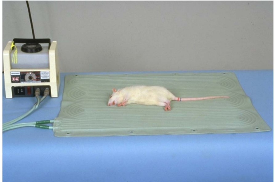
Circulating Water Mat
