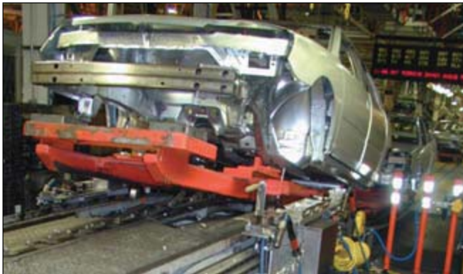
Automotive assembly plant. LoPro is used to carry an air gun and parts for assembly, minimizing the possibility of workers tripping over long hoses and carrying heavy loads.
