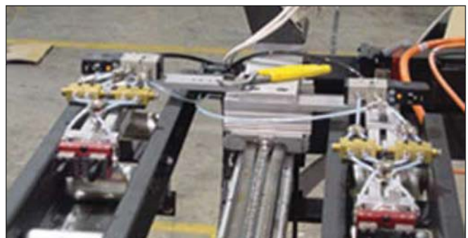
A chain driven LoPro is used on a vinyl fence production machine pushing vinyl fence components into a drill press.
