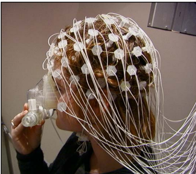
Figure 3.5. Subject wearing the 64-channel EEG net and holding in place the CRO odour delivery and respiratory monitoring mask.
