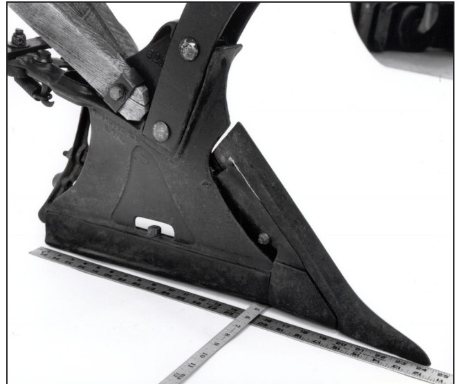
Figure 12—Syracuse plow showing about \frac{7}{8} inch of hillside suction.
