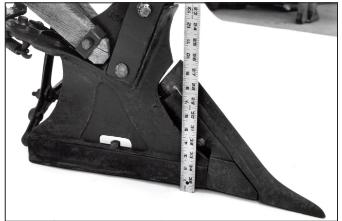
Figure 13—Syracuse plow showing about 1\frac{1}{2} inch of bottom suction.
