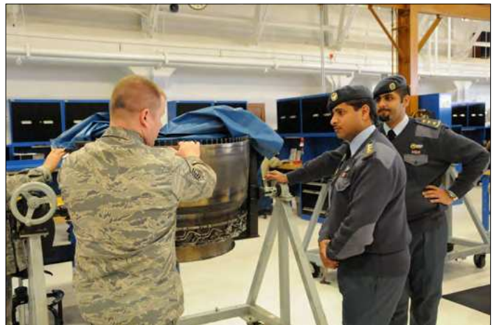
SPRINGFIELD, IL -- Master Sgt. Carl Hasselbring (left) shows Capt. Loay Yusuf Almannaei (middle) and Capt. Ahmed Badia Alsaad (right) of the Royal Bahraini Air Force (RBAF), how custom made aircraft engine component covers reduce the risk of foreign object damage during the engine rebuilding process, during a tour March 6.
