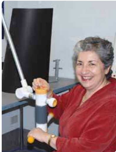
Professor Mary Galea demonstrates the ReJoyce workstation, which patients will operate using a wireless stimulator to make different grasping and releasing hand functions
